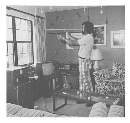
Figure 1. Field intercomparison of passive formaldehyde monitors in house No. 5; the air drift velocity is being measured by observing the drift of smoke powder along a meter stick.
